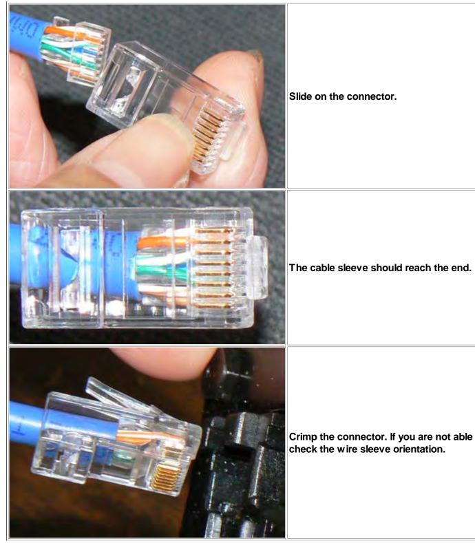
Crimp the connector. If you are not able to crimp, check the wire sleeve orientation.
