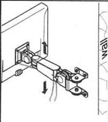
a. Support LCD monitor then slightly move arm upwards & downwards.
