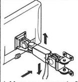
d. Move arm upwards & downwards and make sure knob have wedged into slot. Release support on LCD monitor.
