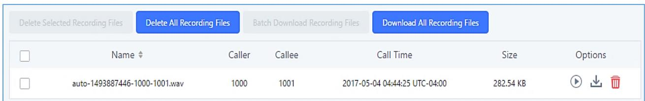
**Figure 235: Download Recording File from Recording Files Page**
