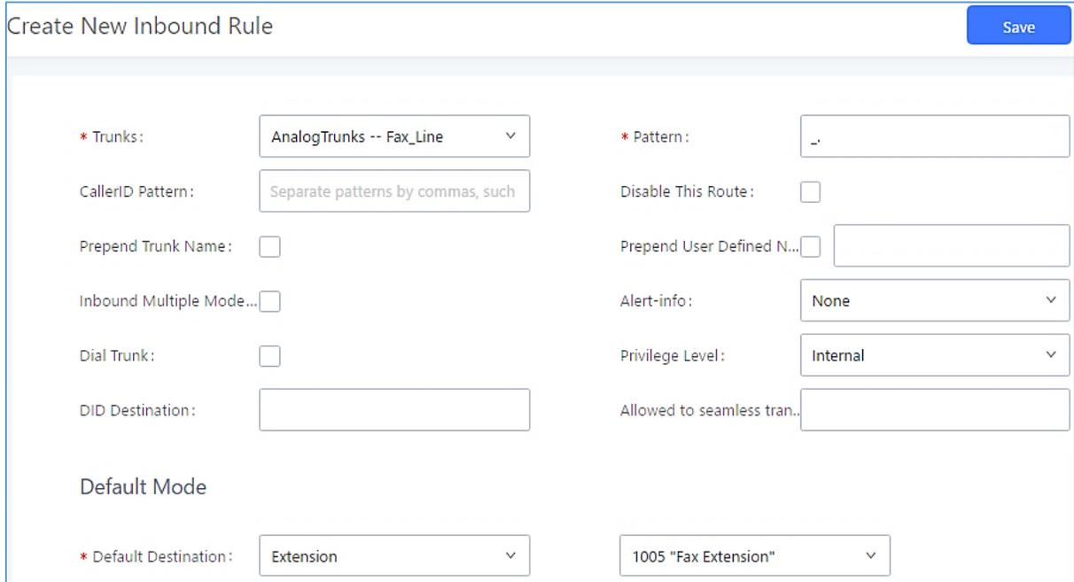
**Figure 204: Configure Inbound Rule for Fax**
