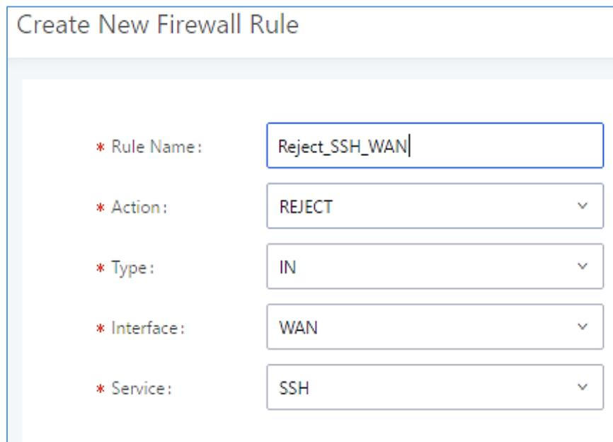
**Figure 28: Create New Firewall Rule**
