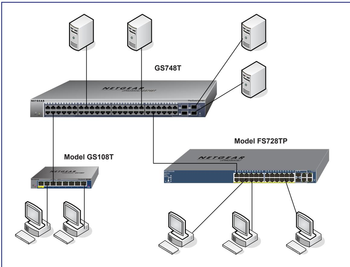
Figure 8. Backbone Switching
