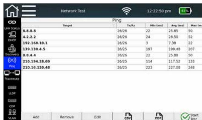
Ping any URL or IP for connectivity testing and perform up to six ping tests simultaneously on the network or internet
