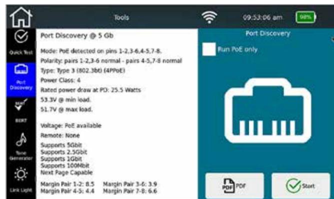
The NetXpert XG2 will test for PoE up to 90W, and displays load, current and voltage, as well as detecting PoE class
