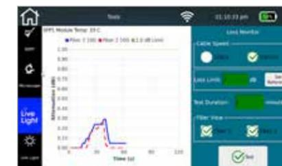
Dirt and debris, bad cable routing, or bad terminations all cause signal loss. LiveLight shows this loss in real time, while microscope inspection clearly shows where cleaning is needed to resolve many connectivity issues.
