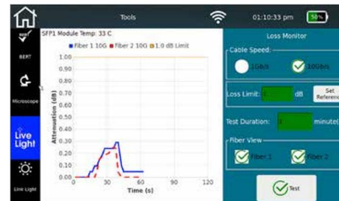
The NetXpert XG2's exclusive LiveLight feature displays fiber signal performance in real time to evaluate cable routing
