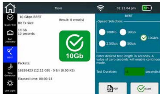
Stress test a network at multiple speeds up to 10Gb with a continuous BERT test of a pre-set duration
