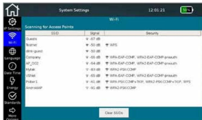
The NetXpert XG2's built-in Wi-Fi detects all networks in range and displays actual signal strength at its location
