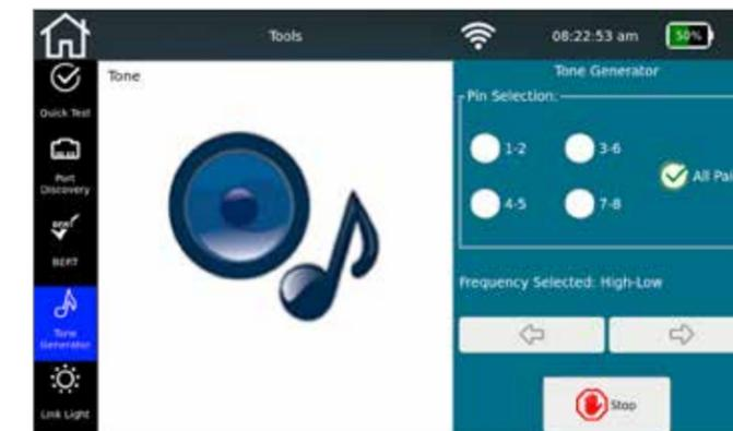
Advanced tone generation over a single pair or all pairs with multiple tone choices for fast, easy cable tracing with a probe
