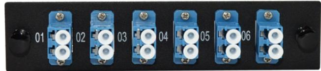
The 6 single mode duplex LC enclosure panel populates open panel slots in compatible wall-mount enclosures and rack trays. The panel is compatible with LGX-118 panel slots and features push-pin style mounting tabs for quick installation.
